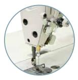
Thread Nipper Device with minimum amount of oil. Oil splashes are now shielded by the frame oil recovery mechanism and automatic oil circulation mechanism above the needle bar.
