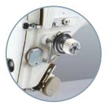
Thread Clamping device
