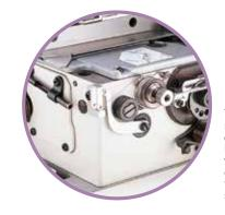
The feed mechanism feeds double chainstitch looper thread with consistency, even under a low tension. (Safety stitch machine)
